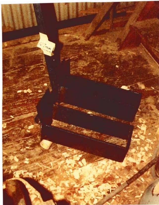
Figure 4a. In an experiment to design chip flow diversion devices for automatic sampling, three widths were tested – 100 mm (not shown), 127 mm and 152 mm (foreground)
