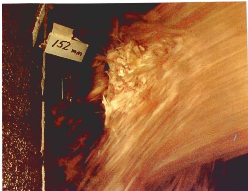
Figure 4b. When held perpendicular to the chip flow, even the largest diverter (152 mm) plugs quickly.
